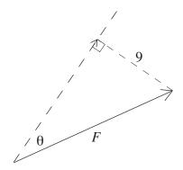
additional information given in the diagram to compute the magnitude of the component of F in the direction  $\theta$ .
