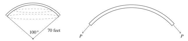
of the shell above the gallery of windows. Using the information in the sketch, the estimate of 23,500 cubic feet for the volume of the original dome, and the weight of the masonry of the shell as 110 pounds per cubic foot, estimate the force P that each of the 40 ribs exerted on the base of the original dome.
