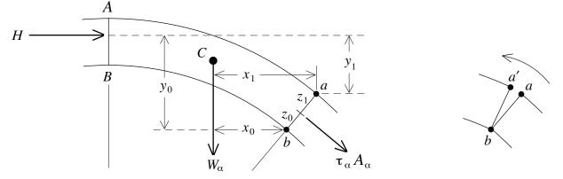
all act on the arch segment ABba. The point C is the center of mass of the segment. Express the torque (rotational effect) of each of the forces around the point b and say whether it is clockwise or counterclockwise. What inequality relating these torques guarantees that hinging failure of the type shown on the right will not occur. Place your inequality in the box below.
