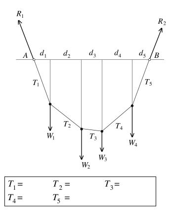
1) Consider the case where the respective magnitudes of the vertical components of  $R_1$  and  $R_2$  are 25 and 35 pounds and the respective magnitudes of their horizontal components are both 30 pounds. The four weights are  $W_1 = 15, W_2 = 20, W_3 = 15$  and  $W_4 = 10$  pounds. Let a vector of length 1 inch represent a force of 10 pounds and draw the force polygon for this situation into the space provided above. Use your diagram to provide close estimates (in pounds) of the tensions:
