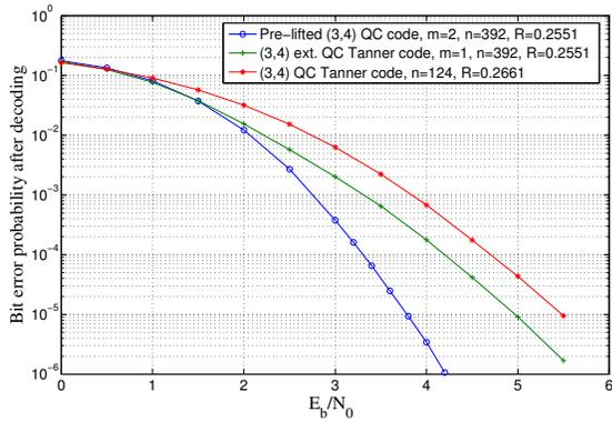
Fig. 1: Simulated decoding performance for the pre-lifted (3,4)-regular QC-LDPC code  $\mathcal{C}_1$  described in Example 2, the extended (3,4)-regular Tanner QC-LDPC code  $\mathcal{C}_2$ , and the original Tanner code  $\mathcal{C}_3$ .
