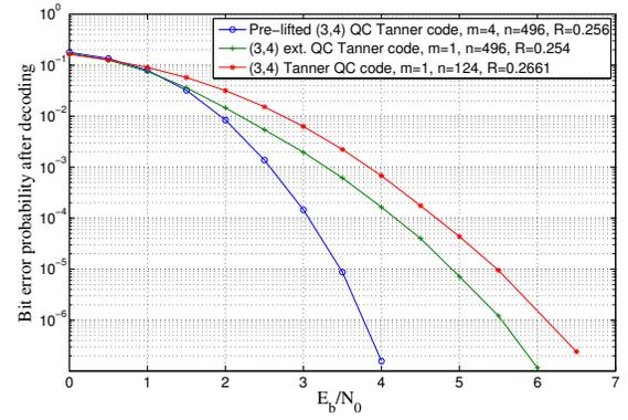
Fig. 2: Simulated decoding performance for the pre-lifted (3,4)-regular QC-LDPC code  $\mathcal{C}_4$  described in Example 3, the extended (3,4)-regular Tanner QC-LDPC code  $\mathcal{C}_5$ , and the original Tanner code  $\mathcal{C}_3$ .
