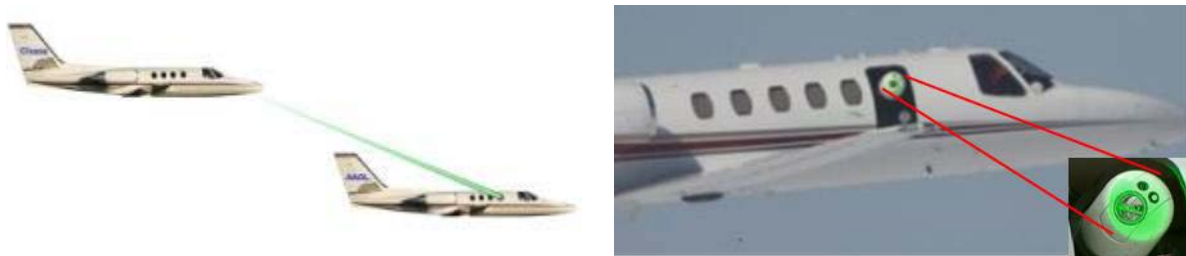
Figure 1: Notre Dame's Airborne Aero-optics Laboratory. Left) Two Citations flying in formation to measure the aero-optics effects of the flow around a turret. Right) Picture taken during the first flight test of the laser on the turret.
