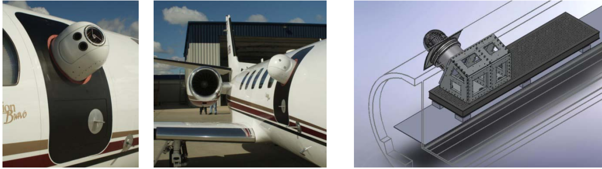
Figure 4: Pictures of the turret mounted on the Citation with a schematic of the turret assembly and shell of the aircraft.
