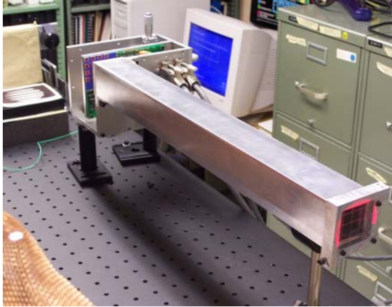
Figure 10. Notre Dame high-bandwidth wavefront sensor: overall view with a box cover removed.
