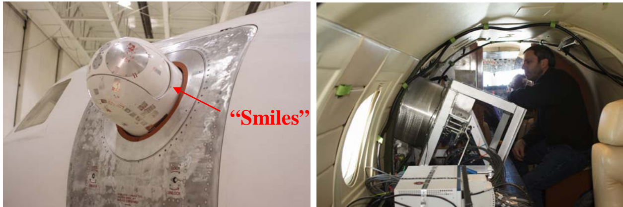
Figure 1: The turret with the conformal window mounted on the AAOL-T, left and the interior testing bench, right.
