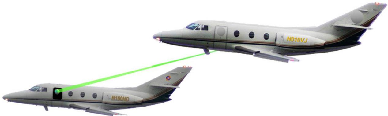
**Figure 3. Schematic of the AAOL-T formation approach with two Falcon 10s flying in formation at a separation distance of 50 m.**
