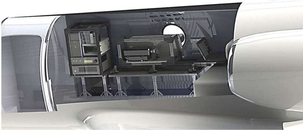
**Figure 10. Rendering of Laser Source Installed in Falcon 10 Showing Sliding Rails, Equipment Mounting and Operator Location.**
