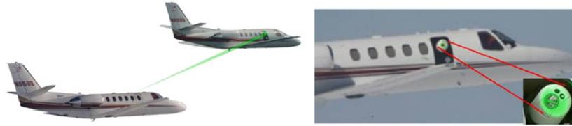
**Figure 4: Picture of the Airborne Aero-Optics Laboratory (AAOL). The pointing aircraft is depicted on the left and the tracking aircraft on the right.**<sup>7</sup>
