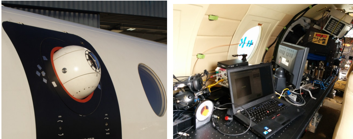
Figure 3: The AAOL turret installed on AAOL-T, left and the instrumented optical bench, right.
