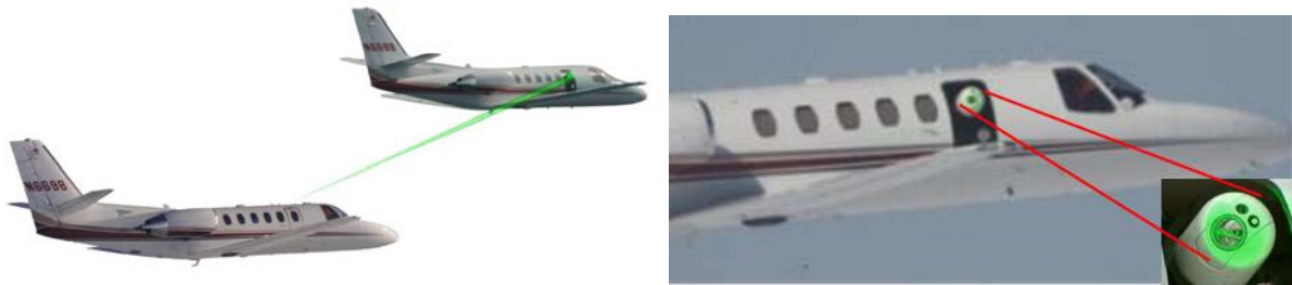
Figure 6: Airborne Aero-optics Laboratory; Left, Schematic of the two Citations flying in formation; Right, Picture taken during a flight test, note laser on the turret.
