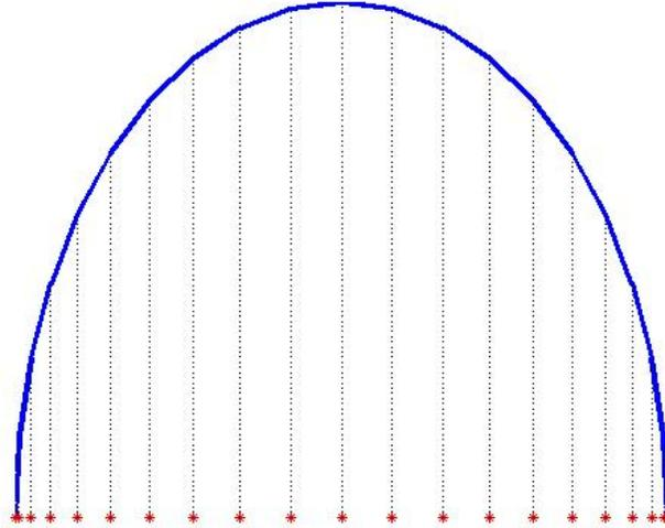
Figure 1: Chebyshev mapping to generate gridpoints in R direction from the unit circle.
