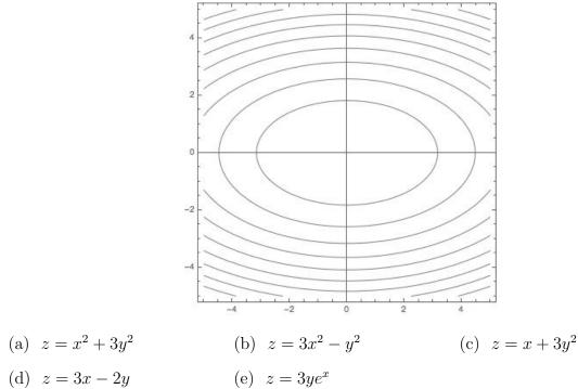
**Solution.** The only answer choice with ellipses as level curves is  $z = x^2 + 3y^2$ . The level curves of  $z = 3x^2 - y^2$  are hyperbolas. The level curves of  $z = x + 3y^2$  are parabolas. The level curves of z = 3x - 2y are lines. The level curves of  $z = 3ye^x$  are exponential functions.
