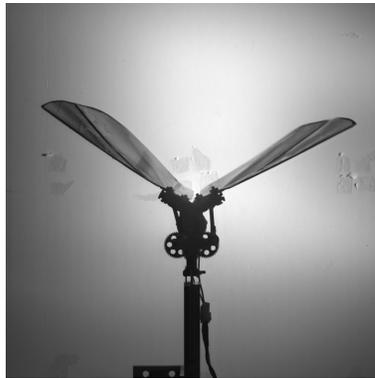
Figure 2.16. One of the frames captured during high speed flapping of the stiff wing
