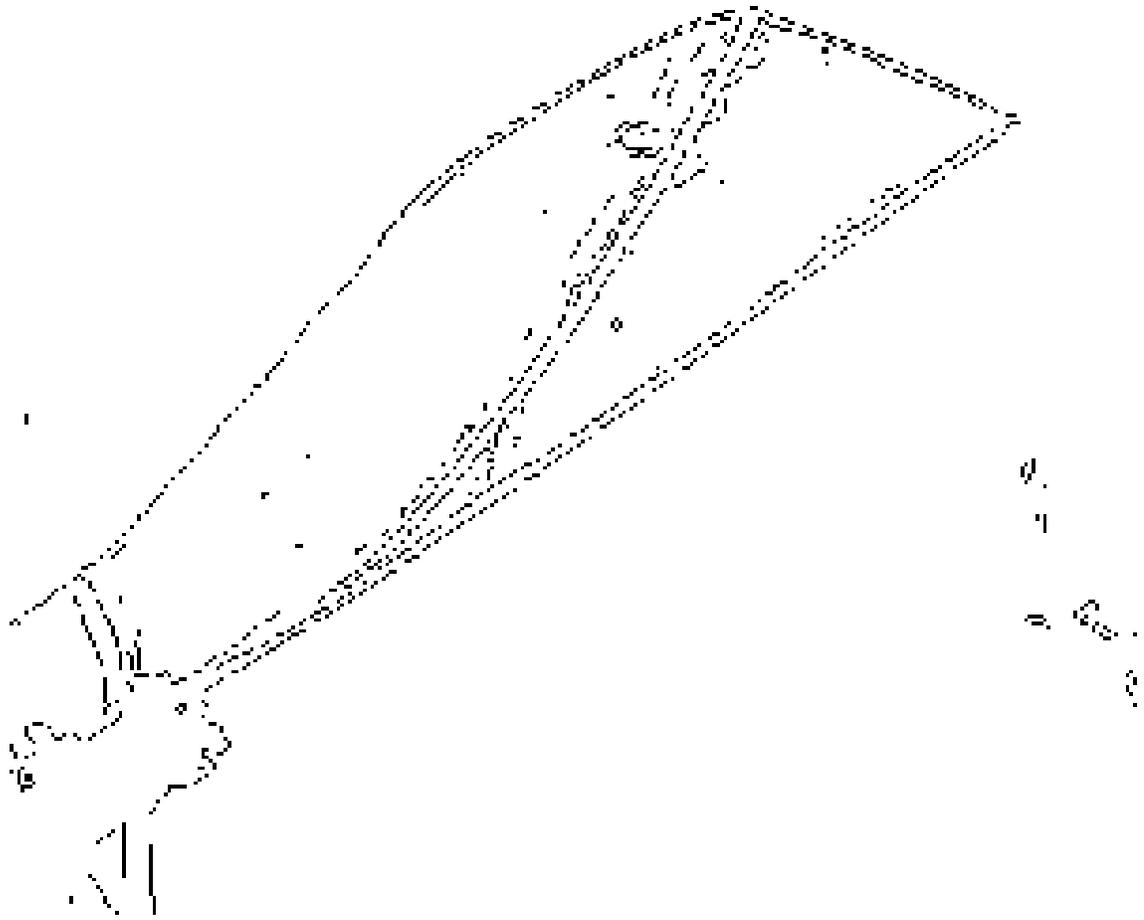
Figure 4.6. The output of the Prewitt edge detection filter for an image of the flexible wing.
