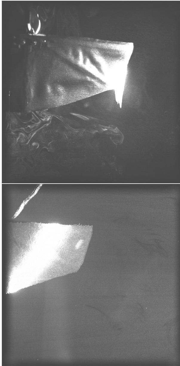
Figure A.5. Images captured by the PIV camera with the laser at low power showing specular reflections off the wing. The top image shows the reflection off black and rhodamine paint, the bottom matte black fabric
