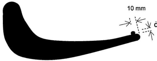
Figure 1.6. The “Langston” blade with a Gurney flap attached to the pressure surface near the trailing edge (from Byerley [4]).
