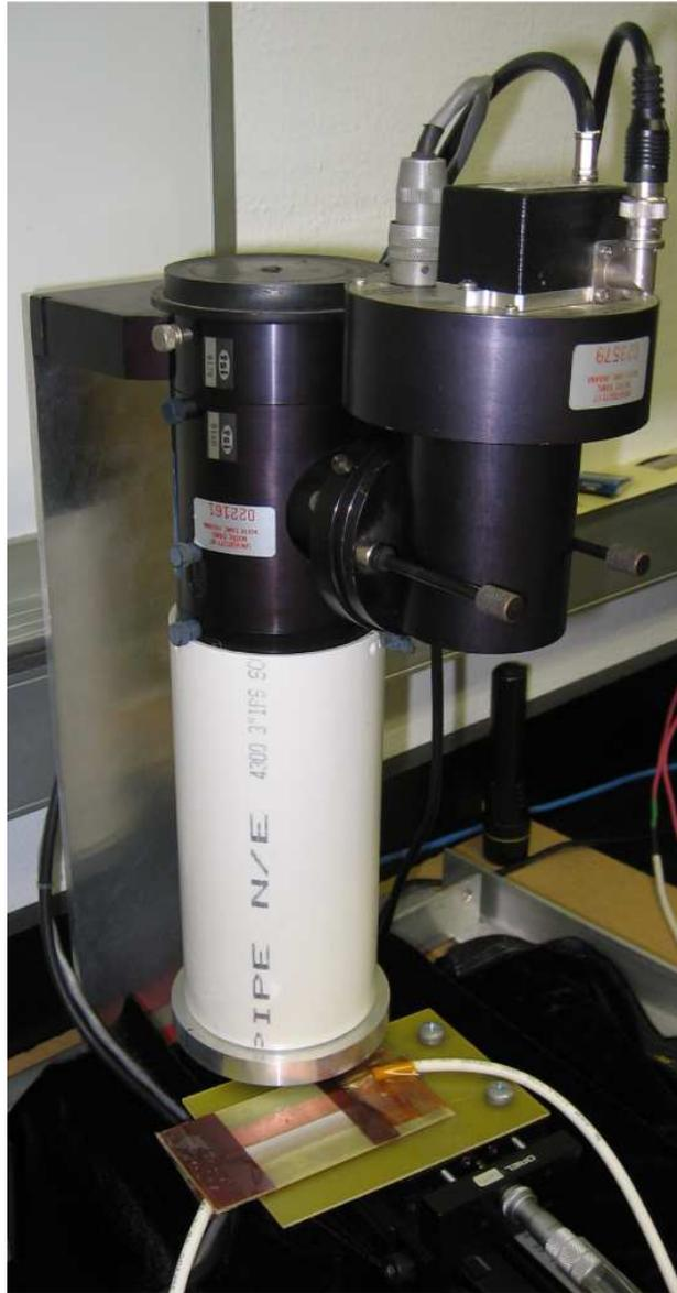
Figure 2.1. Experimental setup used in measuring plasma light emission for SDBD model validation.
