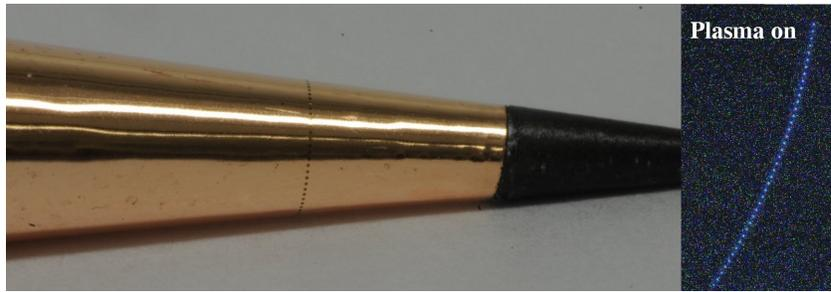
Figure 2.16. 0.5 mil thick Kapton actuator glued to a Torlon carrier cone. Right hand side picture shows the operating plasma dots at 3 inHg ambient pressure with 2.2 kVpp and 3 kHz sin-wave HV
