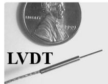
Figure 2.7. LVDT displacement sensor for the wall normal motion of the wedge and Pitot tube.
