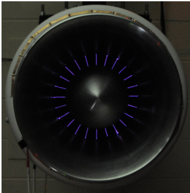
Figure 6: Photograph of operating plasma actuators on the array of 24 3/16 in. diameter cylinders in the circular test section. Note that the cylinders had been rotated 90° towards the test section inlet for the glow to be more visible.
