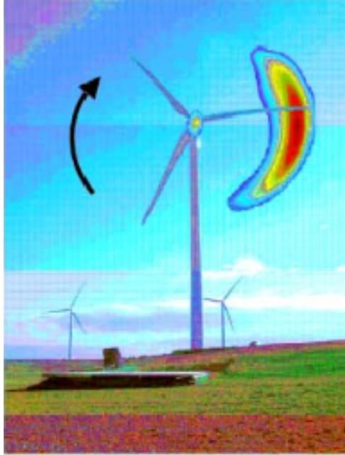
Figure 6: Color rendering of the sound pressure levels obtained with a focused microphone array that pin-point the broadband noise source on the downward moving rotor.
