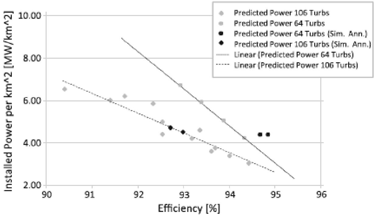
Figure 4: Impact of site area and number of wind turbines on wind farm efficiency.
