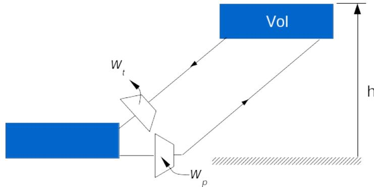
Figure 10: Schematic of a hydro-electric storage configuration.
