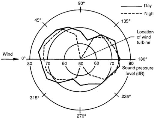
Figure 7: Sound pressure level azimuthal radiation pattern for a wind turbine.
