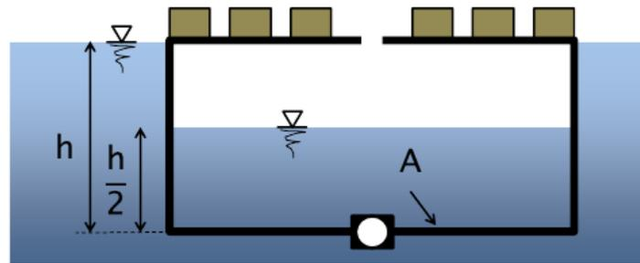
Figure 11: Schematic representation of the buoyant energy storage.
