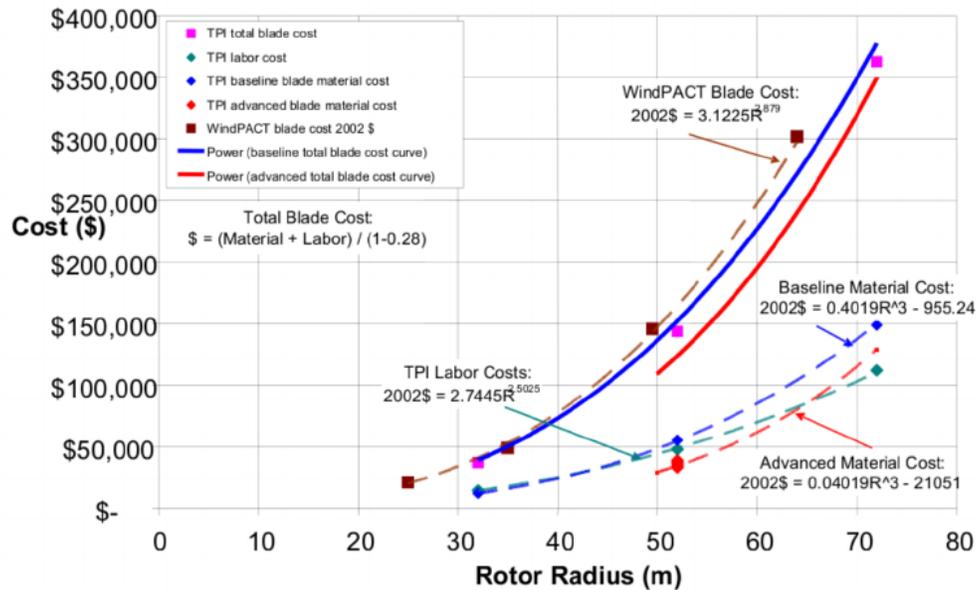
Figure 12: Wind turbine rotor blade cost, labor cost, and baseline and advanced material cost correlations with rotor radius.
