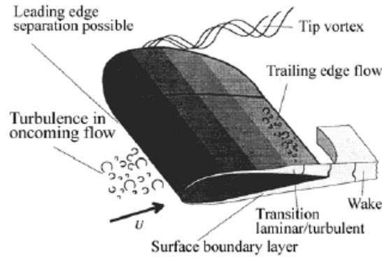
Figure 5: Mechanisms for sound generation due to the air flow over the turbine rotor.
