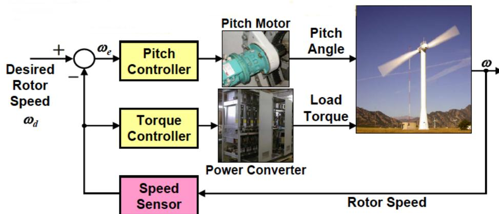
Figure 2: Schematic of a wind turbine closed-loop control system.
