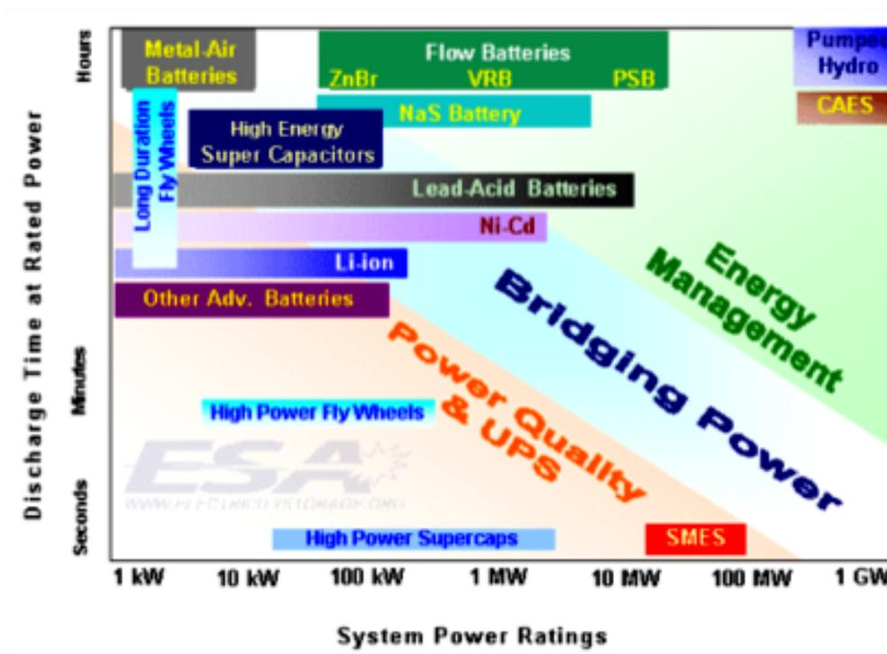
Figure 9: Comparison of different electric power storage systems with regard to power rating and discharge rate.
