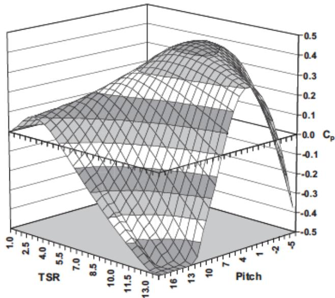
Figure 1: Example of the relation between the rotor tip-speed ratio and rotor pitch angle on the coefficient of power for a 600kW two-bladed horizontal wind turbine.
