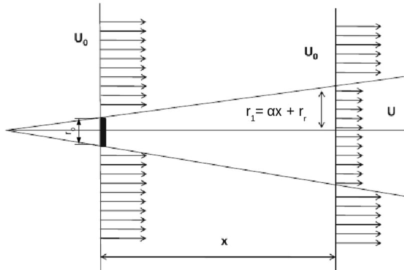
Figure 3: Schematic drawing of wind turbine wake model.
