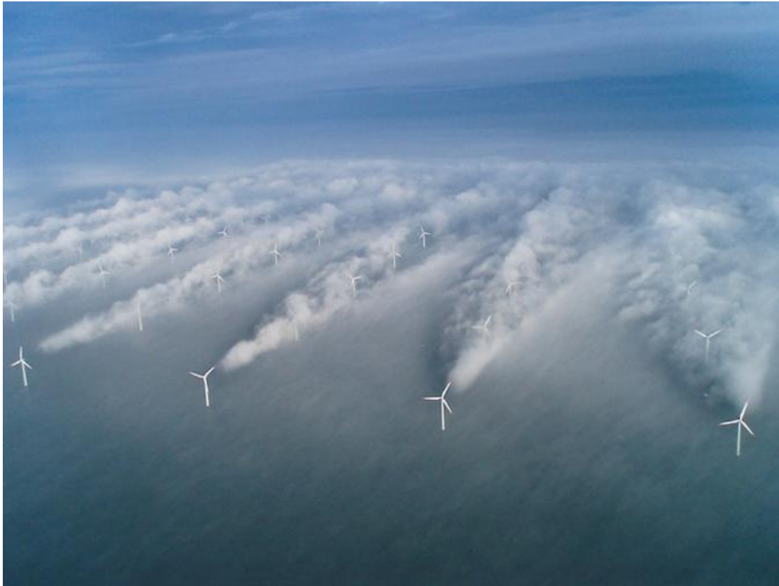
Figure 3: Photograph showing the wakes from wind turbines made visible by low level fog over an an offshore wind farm.
