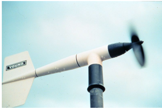
Figure 10: Example of a propeller anemometer that is designed to point into the wind.
