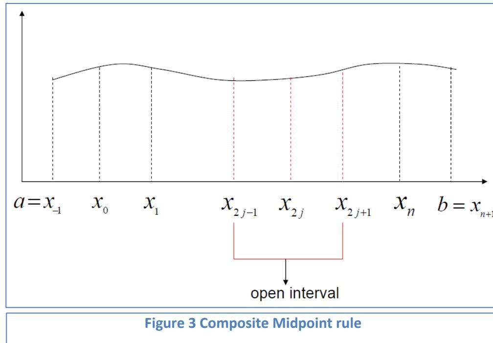
**Theorem 4.6** Let  $f \in C^2[a, b]$ ,  $n$  be **even**,  $h = \frac{b-a}{n+2}$ , and  $x_j = a + (j+1)h$  for each  $j = -1, 0, \dots, n, n+1$ . There exists a  $\mu \in (a, b)$  for which **Composite Midpoint rule** with its error term is
