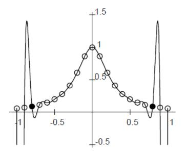
• 21 equal-spaced numbers to interpolate  $f(x) = \frac{1}{1+25x^2}.$  The interpolating polynomial oscillates between interpolation points.
