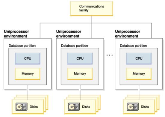
This model assumes that the underlying hardware is a collection of processors, each with its own local memory, and an interconnection network supporting message-passing between processors.
