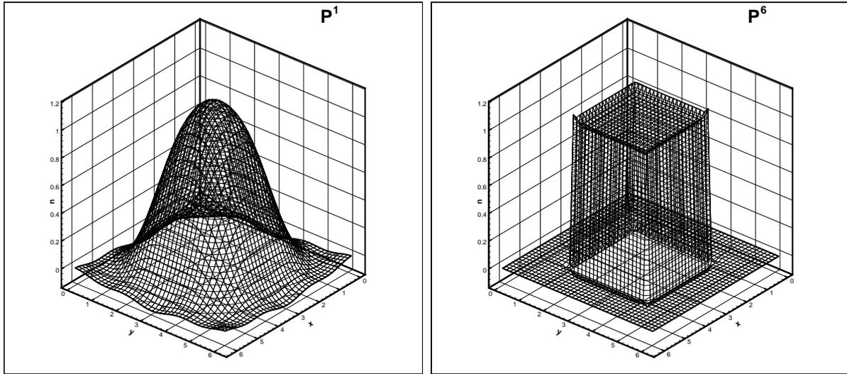
Figure 3.2: Transport equation: Comparison of the exact and the RKDG solutions at  $T = 100\pi$  with second order ( $P^1$ , left) and seventh order ( $P^6$ , right) RKDG methods. Two dimensional results with  $40 \times 40$  cells.
