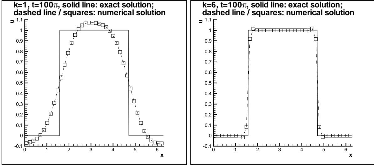
Figure 3.1: Transport equation: Comparison of the exact and the RKDG solutions at  $T = 100\pi$  with second order ( $P^1$ , left) and seventh order ( $P^6$ , right) RKDG methods. One dimensional results with 40 cells, exact solution (solid line) and numerical solution (dashed line and symbols, one point per cell).
