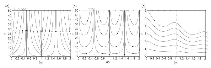
Figure 1. The phase diagrams of second-order LTI systems in polar coordinates: (a) node, (b) saddle point and (c) focus.
