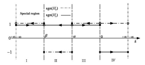
Figure 5.  $S_{11}$ : N(k) has two complex real roots, the switched system is not RAS.
