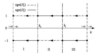
Figure A9.  $S_{33}$ : det( $P_3$ )>0, the best case trajectory rotates around the origin clockwise.
